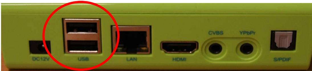
**3.4.5** The remaining USB Port on the **SF-200** can be used for almost any **RS232** controlled devices such as a Commercial Grade Monitor or a **TV One** scaler ([www.tvone.com](http://www.tvone.com)) for example.
