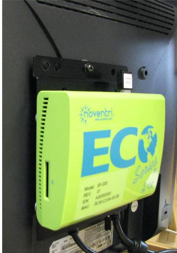
**4.4** Now that the **SF-200** is mounted on the Monitor it is ready to be connected.
