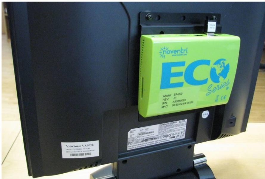
**4.3.3** Mount the assembly to the Monitor using the appropriate hole spacing with two screws.
